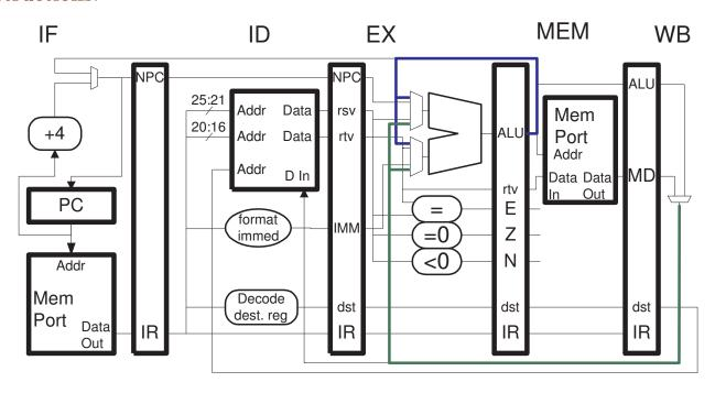
Blue bypass used in cycle 3, green bypass used in cycle 4.
