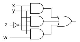
(b) In the expression below xy has been factored out. Draw a logic diagram corresponding to this expression. As far as the diagram is concerned, treat the 1 as an input (x, y, z, and w are the real inputs). Note: If this is solved correctly then something in the diagram should look foolishly wasteful. See the next part.
