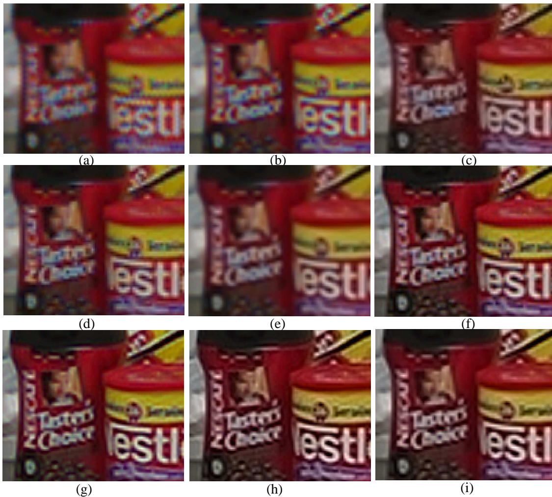
Fig. 11. Demosaicking and super-resolution results. (a) Single frame demosaicking by bilinear interpolation. (b) Single frame demosaicking by edge directed interpolation [Laroche and Prescott, 1994]. (c) Single frame demosaicking by adaptive homogeneity directed interpolation [Hirakawa and Parks, 2005]. (d) Proposed single frame demosaicking by all constraints applied, \sigma_I = 1.41, \sigma_S = 1.41, T_d = 5, T_o = 0, T_c = 2 , domain window is [5 \times 5] , iteration number is 3. (e) Multi-frame demosaicking, all constraints applied. Demosaicking is applied in 3 iterations, \sigma_I = 1.41, \sigma_S = 1.41, T_d = 5, T_o = 0, T_c = 2 , domain window is [5 \times 5] . (f) OSR result using single frame demosaicking in 3 iterations. (g) DSR without consistency set using single frame demosaicking in 3 iterations, T_d = 5, T_o = 0 . (h) DSR with all constraint sets applied in 3 iterations, \sigma_I = 1.41, \sigma_S = 1.41, T_d = 5, T_o = 0, T_c = 2 , domain window is [5 \times 5] . (i) DSR using multi frame demosaicking with all constraint sets applied in 3 iterations, \sigma_I = 1.41, \sigma_S = 1.41, T_d = 5, T_o = 0, T_c = 2 , domain window is [5 \times 5] . Iteration number for super resolution is kept 3 during the experiment.
