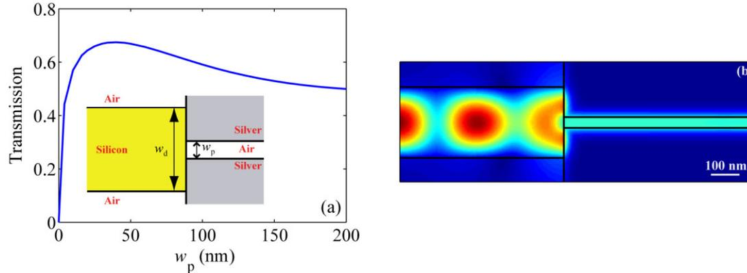
Fig. 1. (a) Power transmission efficiency of a coupler between a dielectric and a MDM waveguide as a function of the width of the plasmonic waveguide  $w_p$  at  $\lambda_0 = 1.55 \mu\text{m}$ , calculated using FDFD. The coupler, created by placing the dielectric waveguide terminated flat at the exit end of the MDM waveguide, is shown in the inset. Results are shown for  $w_d = 300 \text{ nm}$ . (b) Profile of the magnetic field amplitude for  $w_d = 300 \text{ nm}$ ,  $w_p = 50 \text{ nm}$ .
