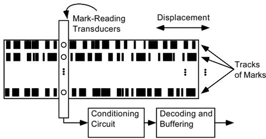
A strip or disk of some material, such as plastic, is mounted on object or on something linked to the object.
