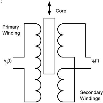
A three-winding transformer with a movable core.
