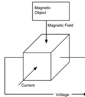
Consists of a block of semiconductor material. There is no PN junction.
