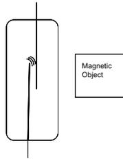
Small glass tube with two switch contacts.
