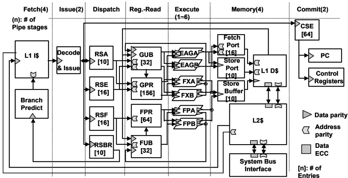
Figure 2. Processor Block Diagram with Error Check Mechanisms
