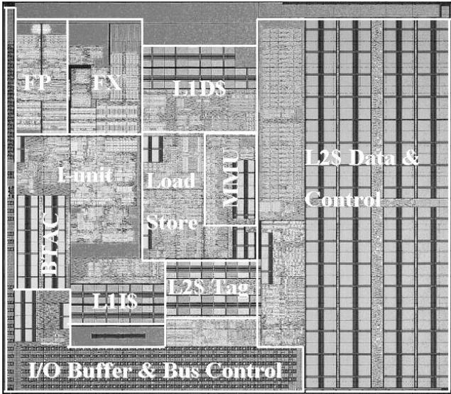
Figure 1. Chip Photomicrograph
