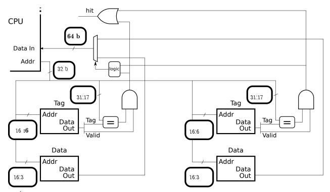
Complete the address bit categorization. Label the sections appropriately. (Index, Offset, Tag.)
