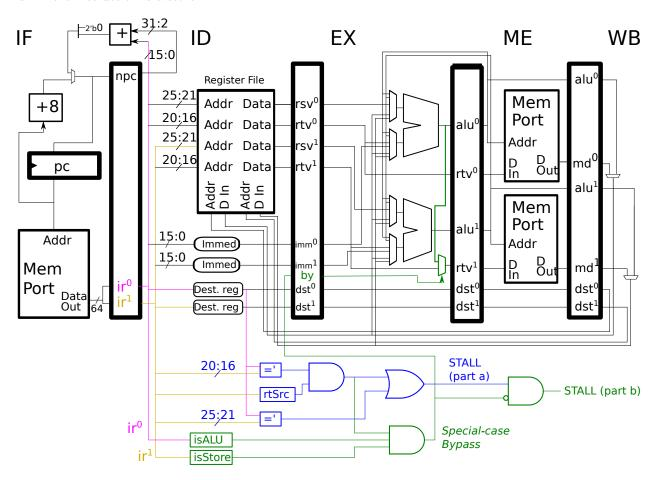
(a) Design logic to generate a signal named STALL, which should be 1 when there is a true (also called data or flow) dependence between the two instructions in ID.
