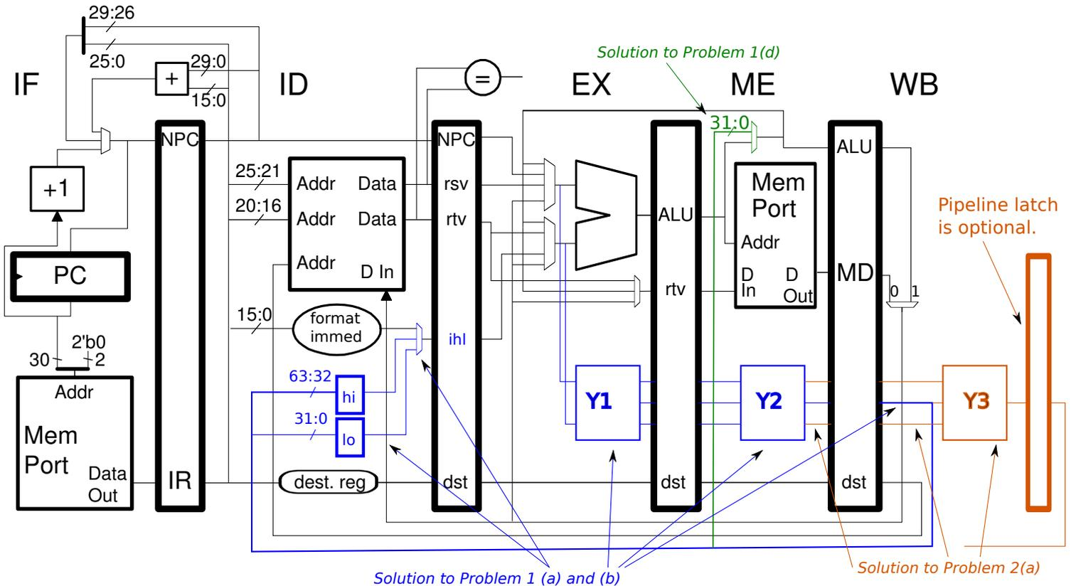
Consider an integer multiply unit that consists of two stages, Y1 and Y2. The inputs to Y1 are the 32-bit multiplier and multiplicand, and the output of Y2 is the 64-bit product. Unit Y1 has three 32-bit outputs named s0, s1, and s2; unit Y2 has 3 32-bit inputs of the same name. As one would guess, the data from the s0 output of Y1 should be sent to the s0 input to Y2, likewise for s1 and s2.
