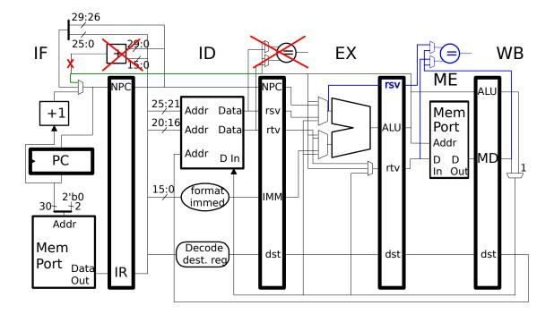
$\checkmark$  Move resolution hardware to the ME stage.
