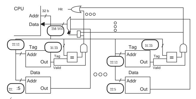
$\bigtriangledown$  Show the address bit categorization. Label the sections appropriately. (Alignment, Index, Offset, Tag.)
