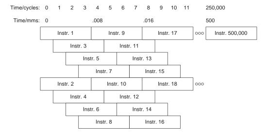
IC = 500,000;  $\phi = 500 \text{ MHz};$  CPI =  $\frac{1}{2}$ .
