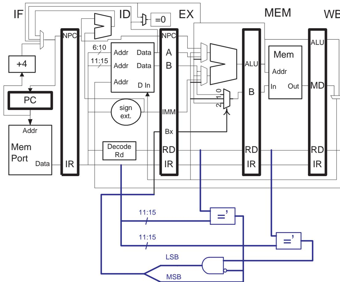
✓ [5 pts] Write a program that uses all three paths into the EX/MEM.B register. *Hint: It's easy.*
