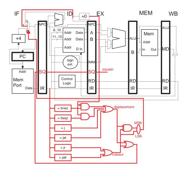
**Problem 3:** How would the hardware designed above have to be modified if DLX had two-slot (yes, two slots!) delayed branches? Jumps still have no delay slots. Ignore interrupts, they will be considered in the next problem.
