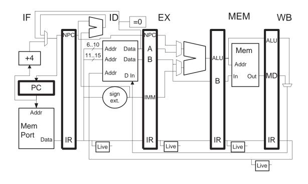
Problem 2: The programs below run on statically and dynamically scheduled systems. All systems are single issue (not superscalar), have perfect branch prediction, have an unlimited number of functional units, and use non-blocking caches. The programs run for a large number of iterations, and the first 1w in every iteration will miss the cache. On a cache miss data arrives 10 cycles after MEM or L2 is entered. The line size is 1024 characters.
