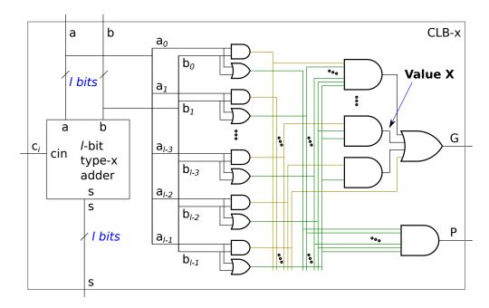
(a) The output of one of the AND gates is labeled Value X. Suppose l = 16. Find inputs to the module such that Value X is 1 but all of the other inputs to the generate OR gate are 0.
