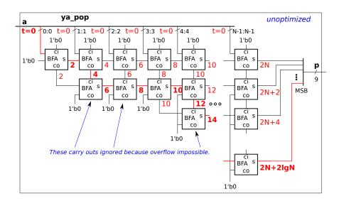
Next notice that the critical path flows through the bottommost BFAs (the delay is shown in red numbers, critical path delays are **bold red**). The path flows through N BFAs to the right and  $\lg N$  BFAs in the down direction, for a total path length of  $N + \lg N$ . The delay is 2 units through each BFA, for a total delay of  $2(N + \lg N)$ .
