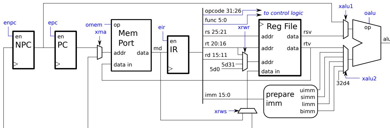
(b) Appearing below are the control signal settings needed to implement the **add** instruction for the VS MIPS presented in class. Show a similar table for the **sll** (shift left logical using **sa** for shift amount) instruction and **srlv** (shift right logical using **rs** register for shift amount) instructions. Insert columns as needed. No need to copy IF and any other unchanged states.
