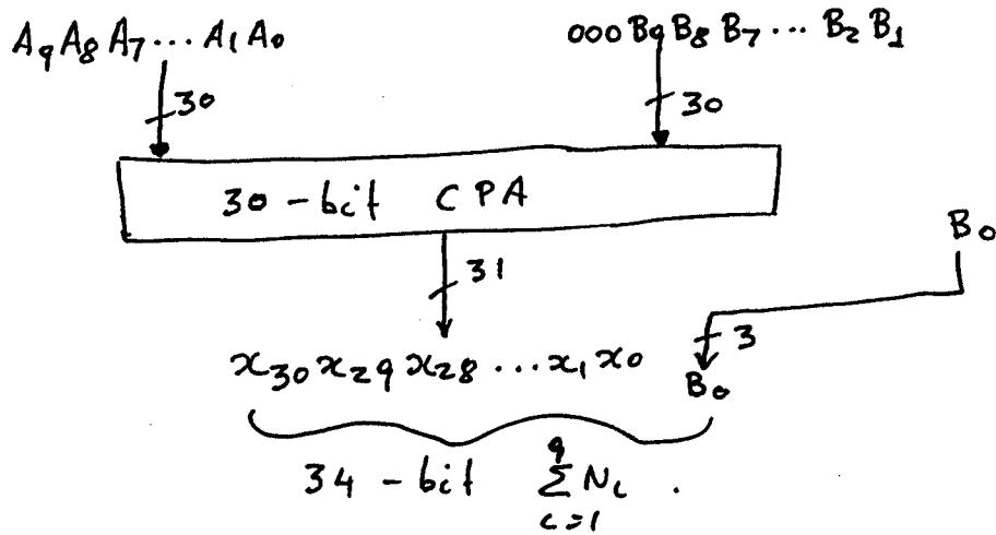
Problem 2: Define the Type I component to be a 3d component that adds 32 2-bit unsigned numbers and produces their full precision summation. Using only Type I components and CPAs (carry propagate adders) show how you can construct an adder capable of adding 32 10-bit unsigned numbers to produce their full precision summation.
