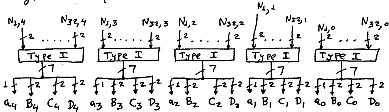
Each Type I component has a 7-bit output since the worst case summation of 32 2-bit unsigned numbers is  $32 \times (2^2 - 1) = 2^5 \times (2^2 - 1) = (1100000)_2$ . (4)d
