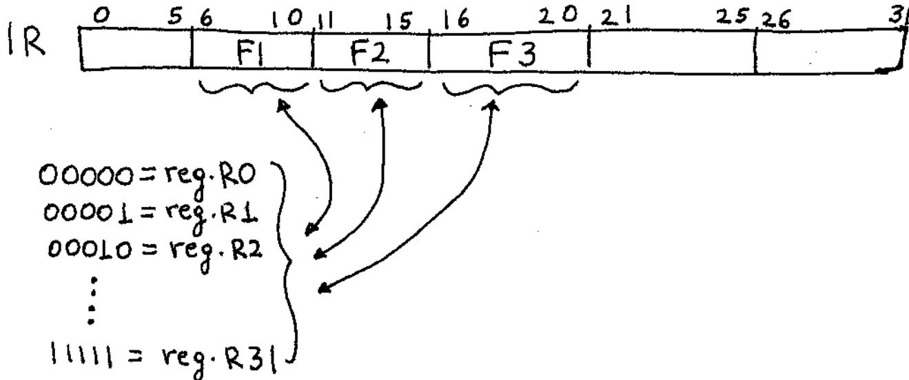
Meaning: Register specified by field F3 is set to 1 if the value in the register specified by field F1 is less than the value in the register specified by the field F2. Otherwise, register specified by field F3 is set to 0.
