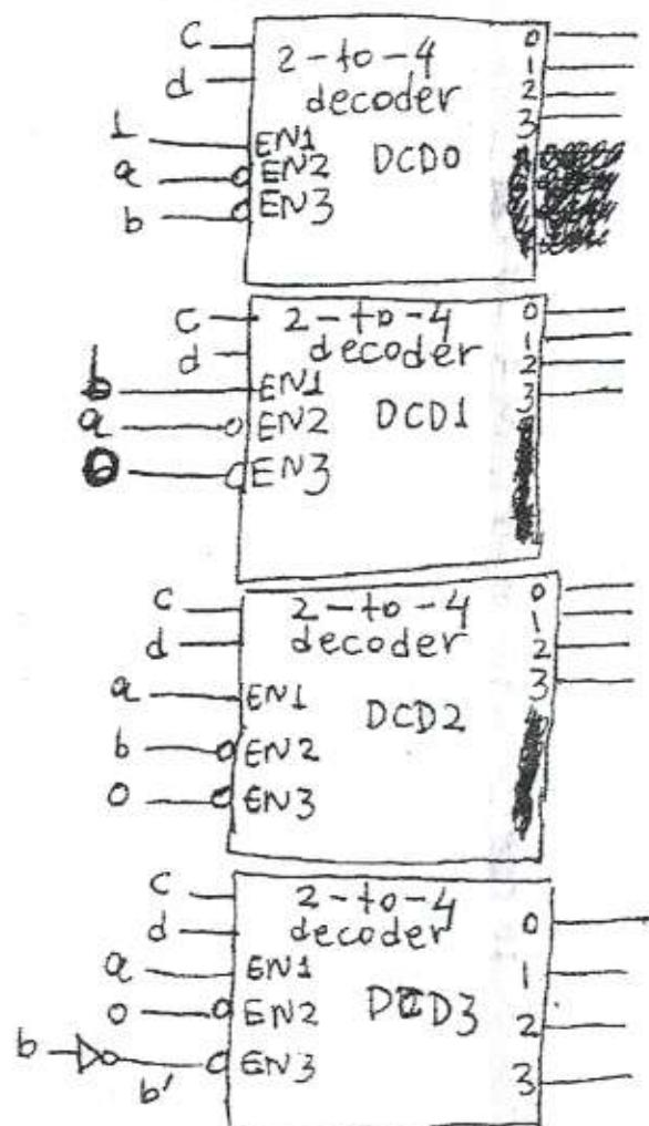
For this 4-to-16 decoder,  $a$  is the MSB of the decoded vector while  $d$  is the LSB of the decoded vector.
