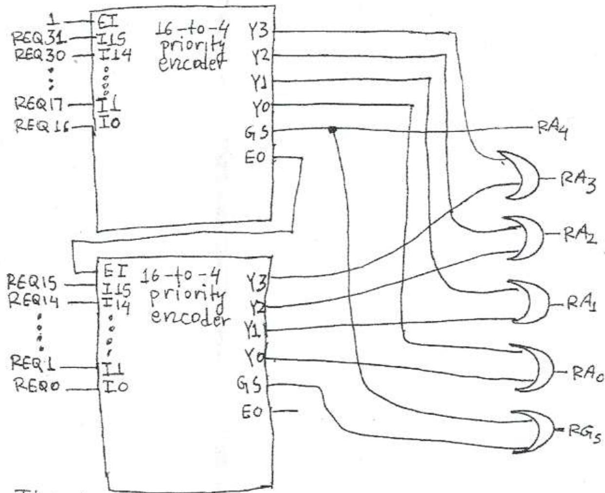
The above figure shows the 32-to-5 priority encoder. Its data inputs are REQ31, REQ30, ..., REQ1, REQ0. The input REQ31 is the highest priority input, while REQ0 is the lowest priority input. Its data outputs are RA4, RA3, RA2, RA1, RA0 with RA4 being the MSB, while RA0 being the LSB. For further explanations, see handout # 19 (following fig. 2 of handout # 19).
